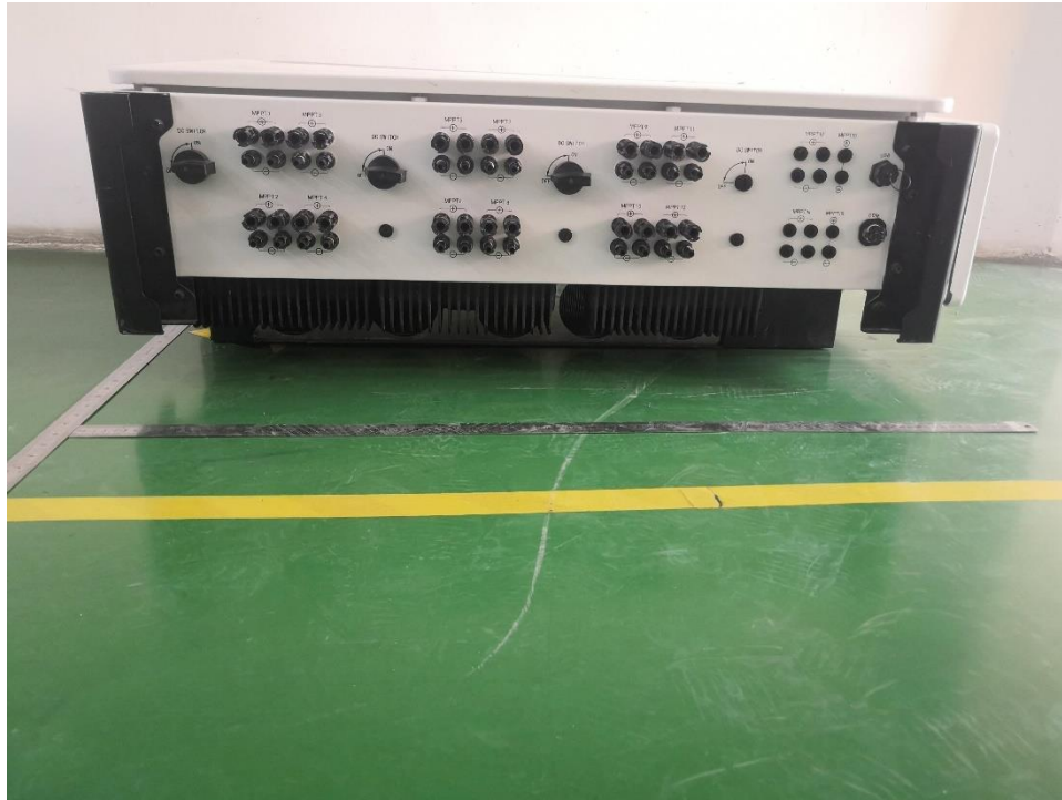
Figure 5. Connection view for MAX 225KTL3-XHV, MAX 250KTL3-XHV
