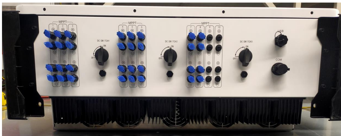
PV Input Terminal view
