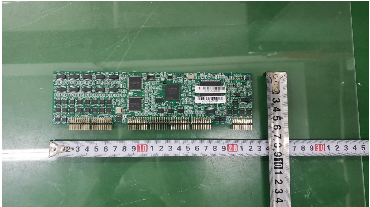
Figure 19. Front view of Control board
