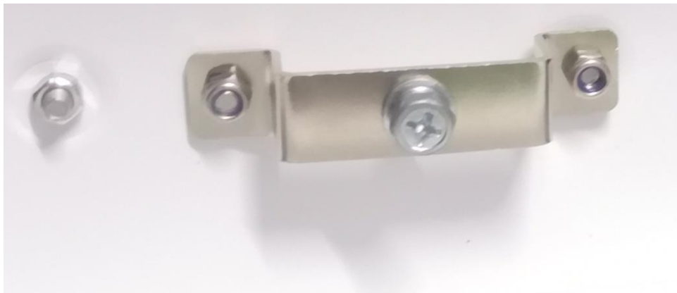
Figure 38. PE terminals view
